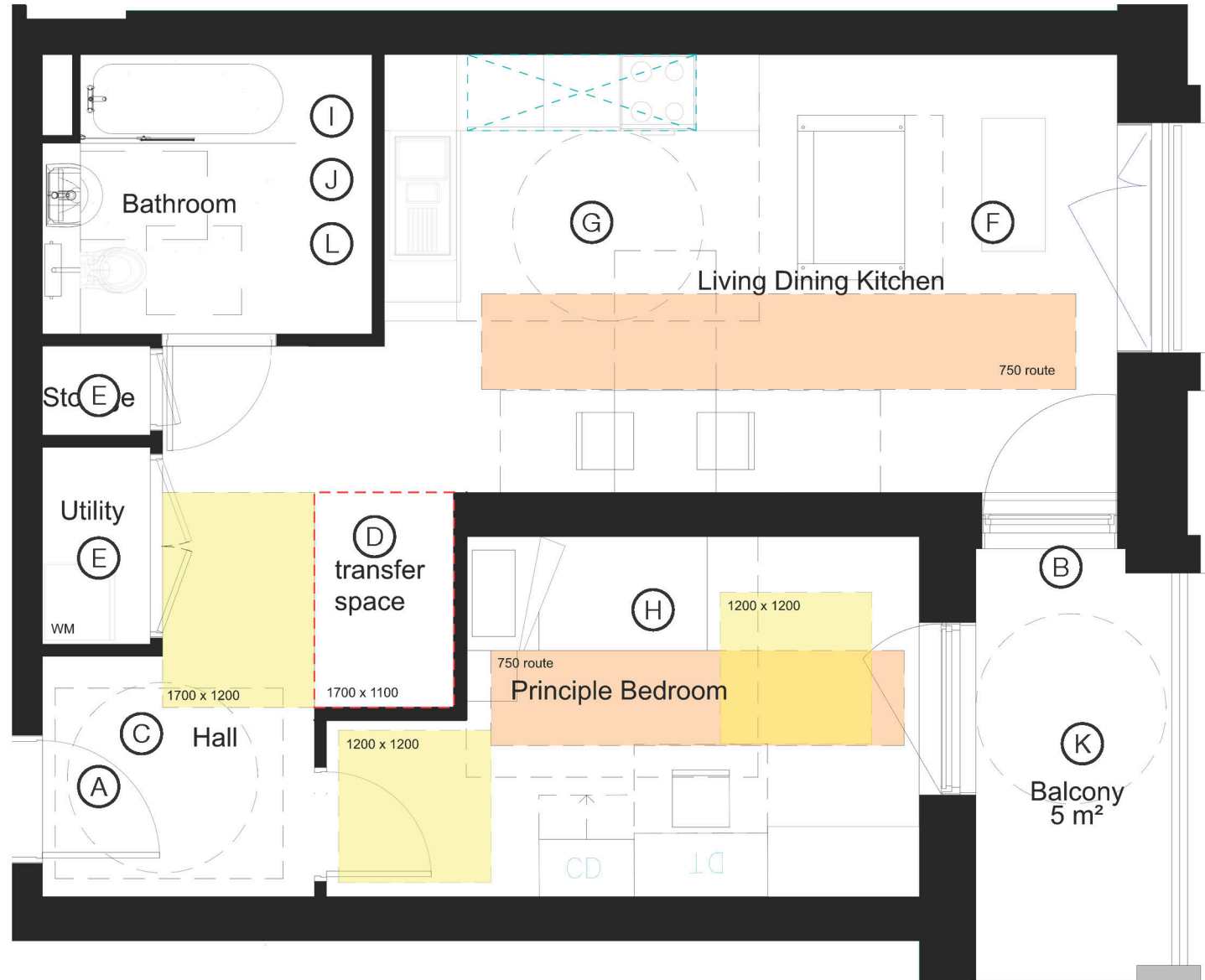
Block H6: 1B/1P Plan - M4(3) Adapted Plan Layout with illustrative letters demonstrating M4(3) provision for Wheelchair Adaptable units.
